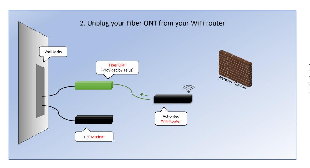
An Optical Network Terminal (ONT) is the device that a fiber line terminates into, and converts optical data into ethernet-protocol data.
