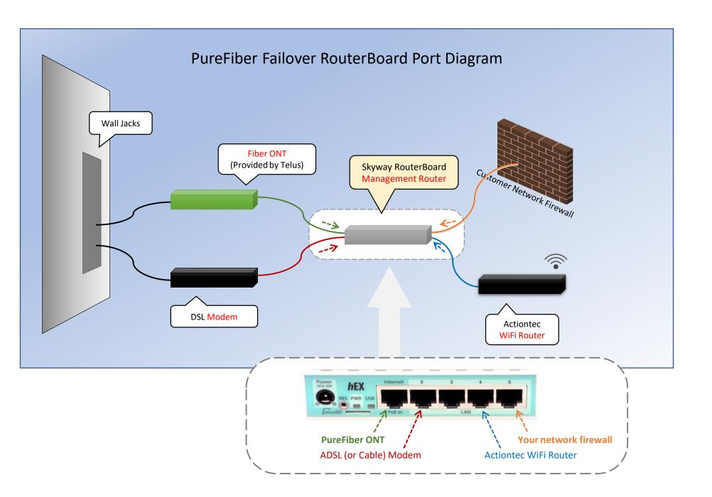
Plug the Fiber ONT into port **ONE** (Internet / PoE port) of the Skyway RouterBoard.
