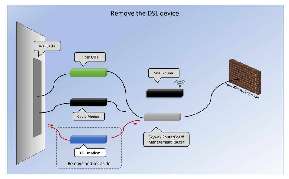
4. Once connectivity has been established on the Fiber ONT, unplug the DSL and remove it entirely from your setup and set it aside (to be returned)
